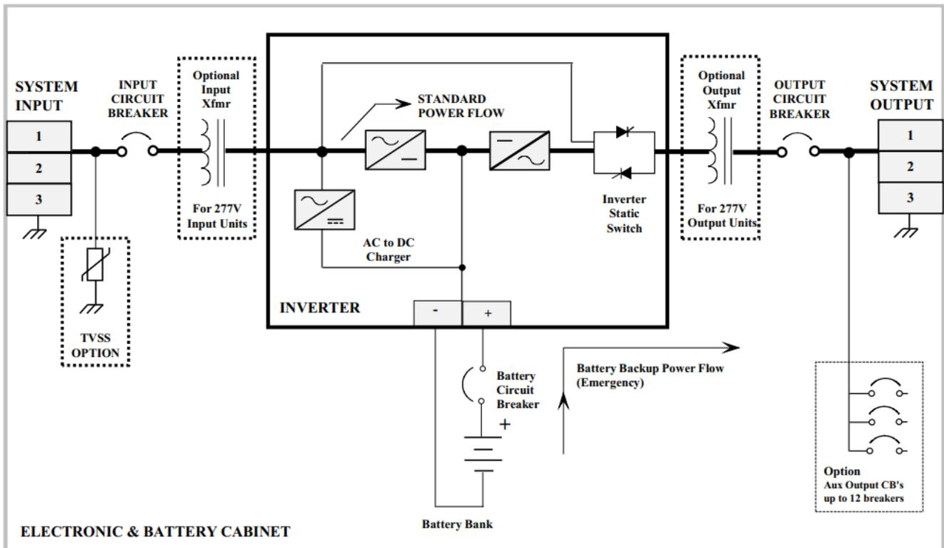
Figure 1-1. Econosine 2 Single Line Diagram (typical)
