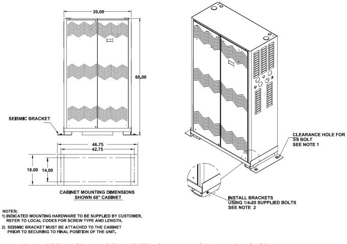
Figure 4-5 Typical Battery Cabinet (8 KW only) Access and Mounting Standard Series (with Optional Zone 4 Seismic Brackets)
