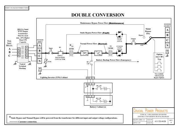
Figure 3-3 System Blocks Diagram (Delta input)
