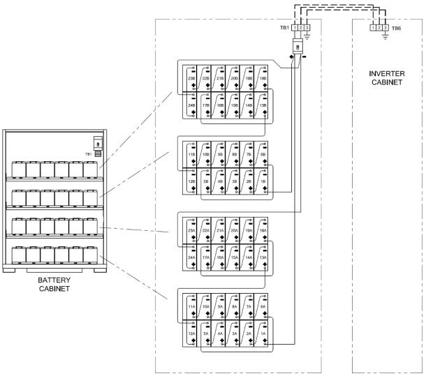
288-Volt Nominal DC Voltage,2 Strings of 24 Batteries (1 cabinet, size: 51" x 70" x 30.5") <u>Typical</u>
