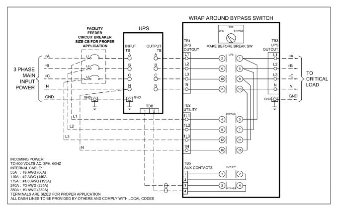
Figure 8-1 External Wrap-around Manual Bypass Switch (same Input and Output Voltage connection diagram (Typical)
