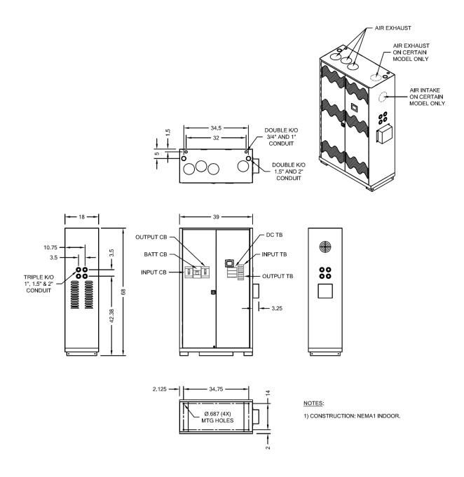
Figure 4-1 UPS Cabinet (8 ~ 50 KW) Access and Mounting (Standard Series)
