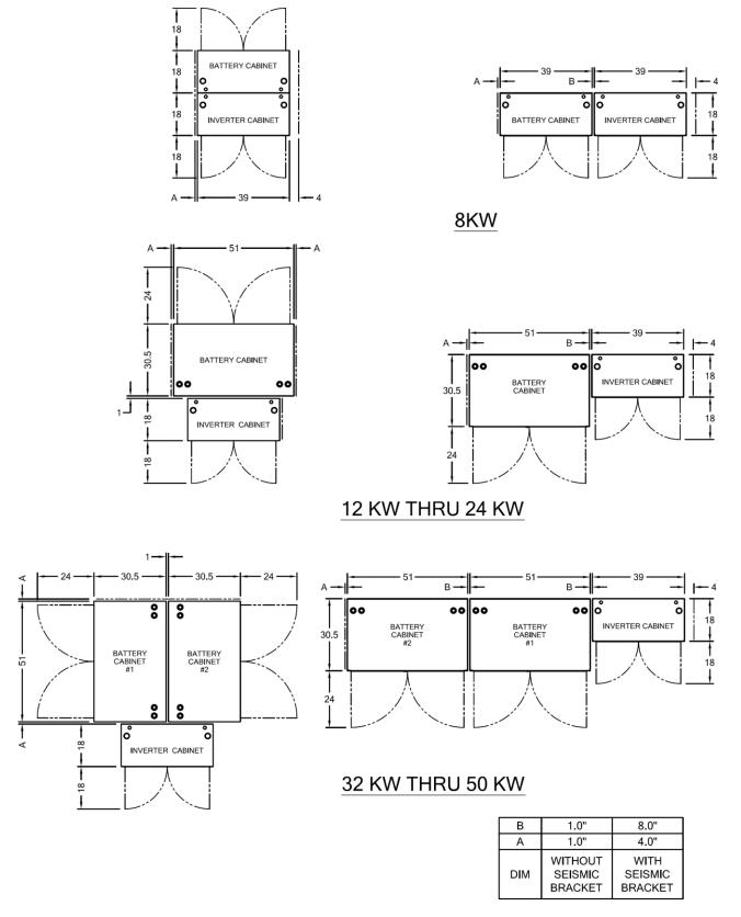
Figure 4-10 Typical system layout (with or without zone 4 seismic bracket)
