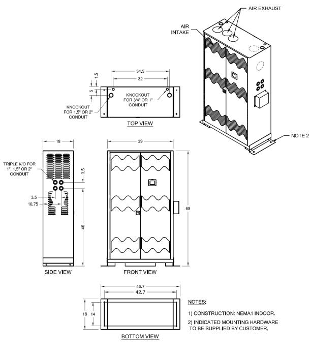
Figure 4-4 .UPS Cabinet (8 ~ 50 KW) Access and Mounting Standard Series (with Optional Zone 4 Seismic Brackets) Installation
