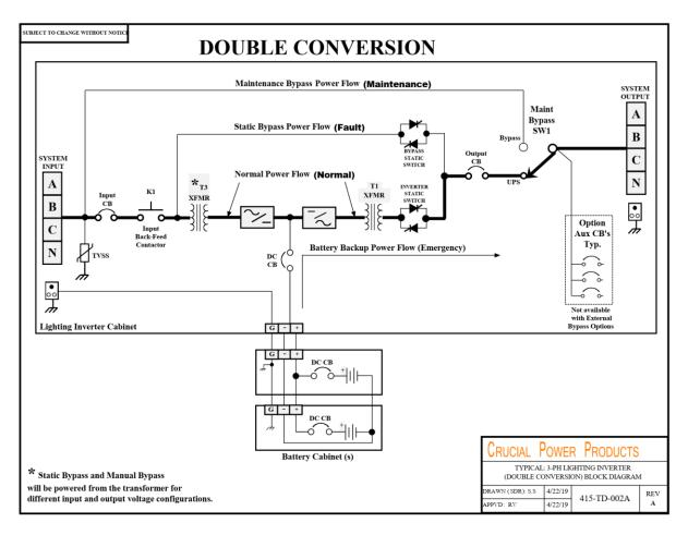
Figure 3-2 System Blocks Diagram
