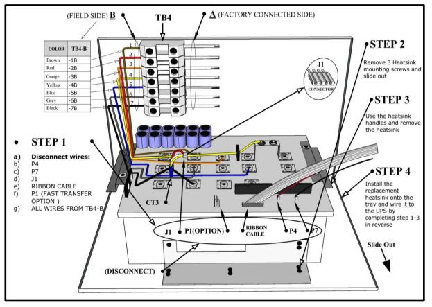
Figure 6-1 Heat sink assembly (10KVA ~ 40KVA)
