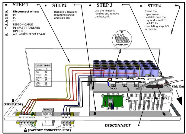
Figure 6-2 Heat sink assembly (50KVA ~ 50KW)
