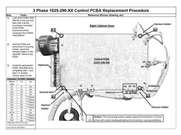
Figure 6-3 Control Board (standard)
