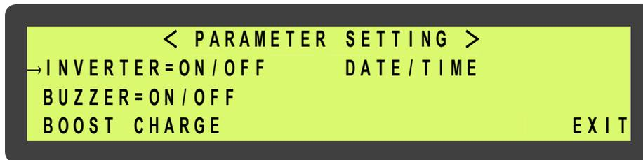
This menu is displayed when < PARAMETER SET > is selected from MENU 1, and the correct password has been entered. The cursor (→) is used to select the parameter the user wants to set, e.g., INVERTER ON/OFF, BUZZER ON/OFF, BOOST CHARGE, DATE/TIME etc. The cursor (→) can be moved upward by the UP (↑) key and can be moved downward by the DOWN (↓) key. The selection is confirmed by pressing the ENTER (←↓) key.
