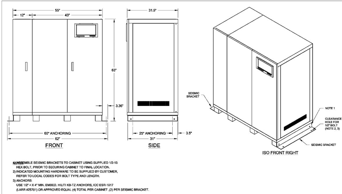
*Figure 4-8 UPS Cabinet (80 ~ 160 KVA) Access and Mounting (with Optional Zone 4 Seismic Brackets)*
