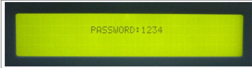
The password is a 4-digit number which can be changed upward or downward by the UP (↑) or the DOWN (↓) key and can be confirmed by the ENTER (↵) key. The selection will continue if the correct password is entered, or will go back to MENU 0, the MAIN MENU, if no correct password is entered after 3 trials. The password for entering the < PARAMETER SET > menu is 1-2-3-4.
