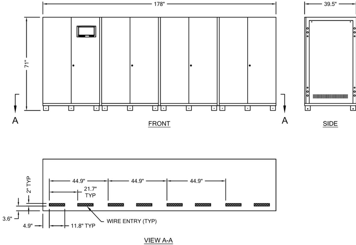
*Figure 4-5 UPS Cabinet (500 KVA) Access and Mounting*
