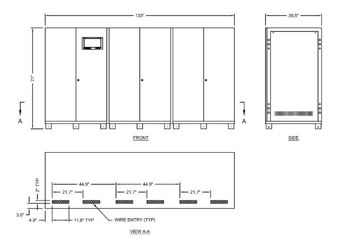
Figure 4-4. UPS Cabinet (400 KVA) Access and Mounting
