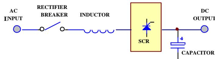
*Figure 1-5 6-Pulse full control rectifier*
