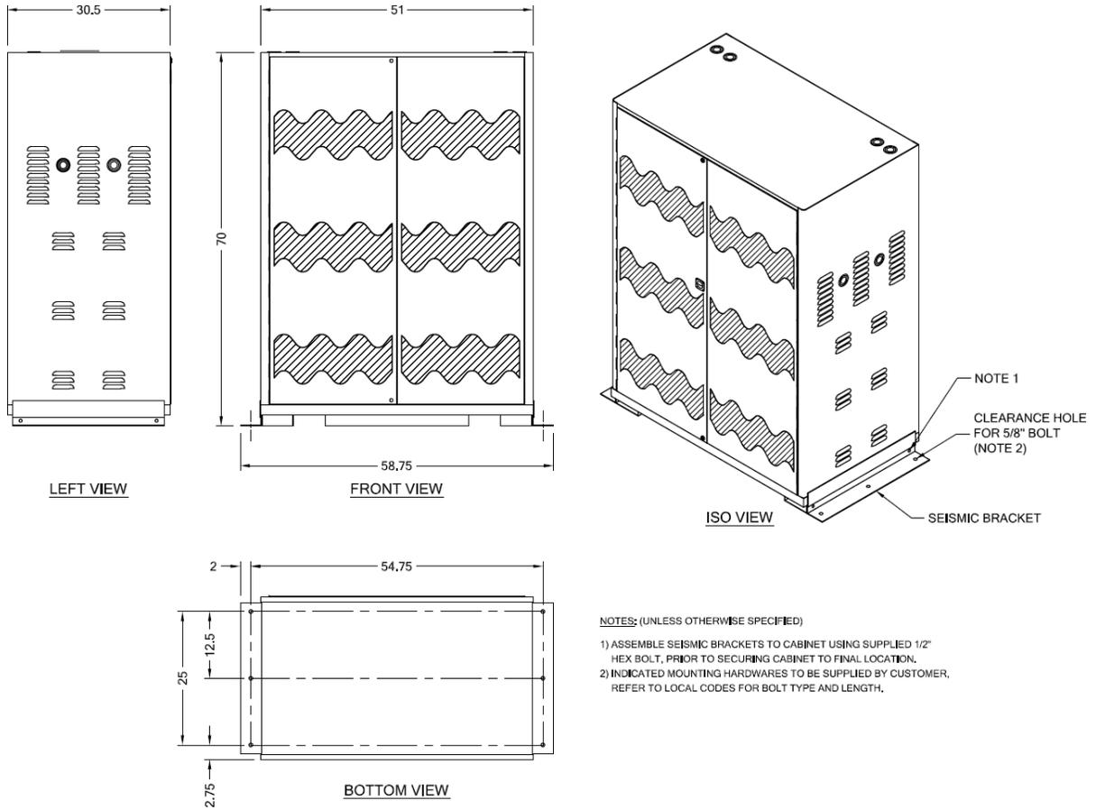
*Figure 4-11 Typical Battery Cabinet Access and Mounting (with Optional Zone 4 Seismic Brackets)*
