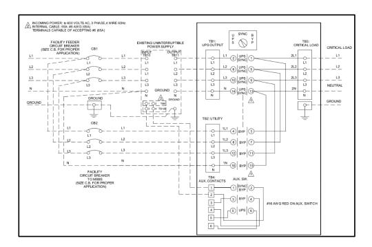
Wrap around Bypass Switch Diagram (Typical)
