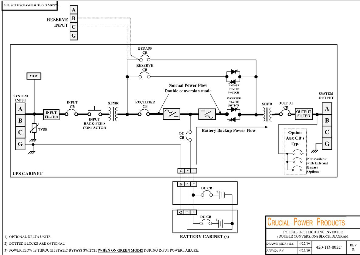
Figure 3-4 System Blocks Diagram (Dual DELTA input power)
