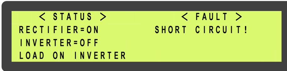
The inverter should be shut off under a short circuit condition. Since the CPU will detect a short circuit, and in order to avoid unnecessary tripping and damage to the breaker, the static switch remains connected to the inverter (will not transfer to reserve).
