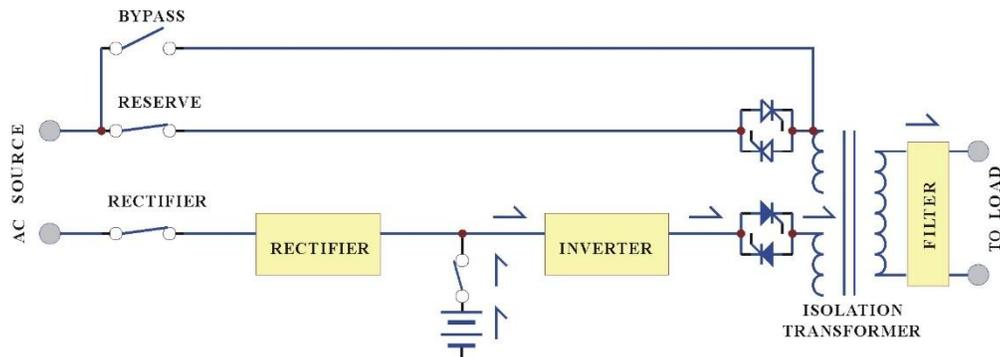
Since the batteries are connected directly to the DC bus, when the AC fails, the batteries change immediately from receiver to donor, supplying energy to the inverter instead of receiving energy from the rectifier. The output AC is not interrupted. Therefore, the load connected to the output is protected.
