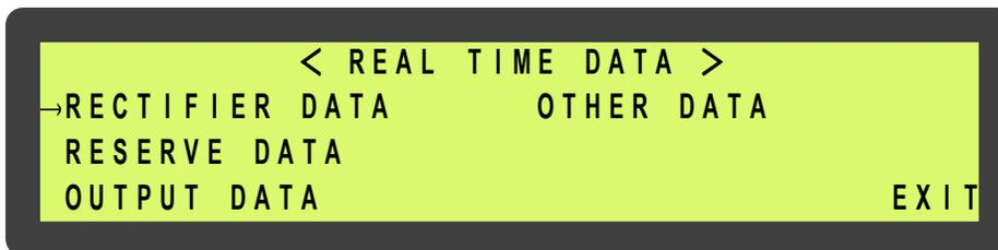
This menu is displayed when the REAL TIME DATA is selected from MENU 1. The cursor (→) is used to select the type of real time data the user wants to view, such as, RECTIFIER DATA, RESERVE DATA, OUTPUT DATA, OTHER DATA etc. The cursor (→) can be moved upward by
