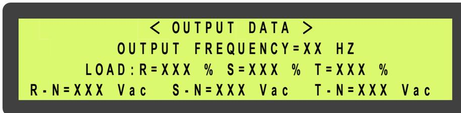
This menu is displayed when <OUTPUT DATA> is selected from MENU 3 – the REAL TIME DATA MENU. It is a data display menu, which shows real time data on the output and load, such as,
