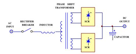
Figure 1-6 12-Pulse full control rectifier
