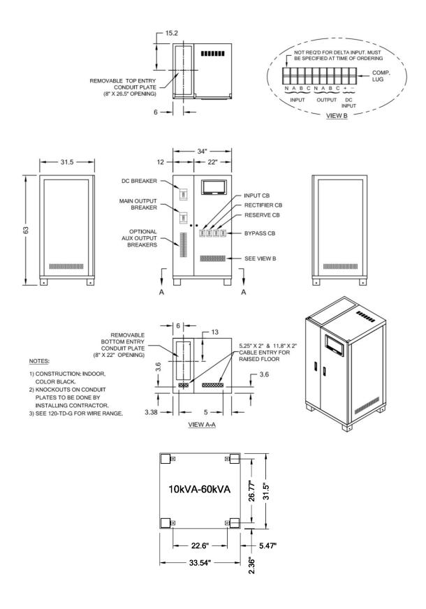
Figure 4-1 UPS Cabinet (10 ~ 60 KVA) Access and Mounting
