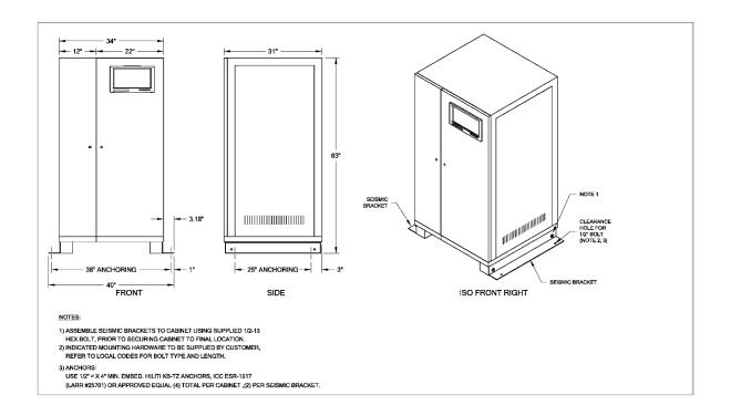
Figure 4-7 UPS Cabinet (10 ~ 60 KVA) Access and Mounting (with Optional Zone 4 Seismic Brackets)
