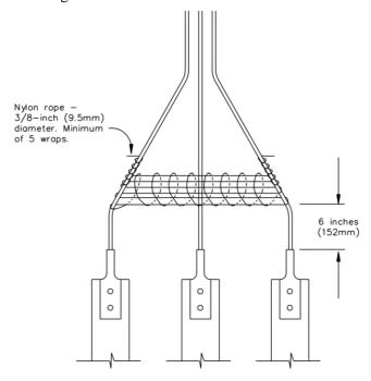
Figure 8-1 Power securement requirement
