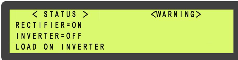
This menu is displayed when STATUS/WARN/FAULT is selected from MENU 1. The left-hand side of this menu shows the real time status of the rectifier, inverter and static switch. The right-hand side shows the warning or fault conditions, if any. Therefore, under normal conditions, the LCD display should be exactly as shown above. When minor abnormal conditions occur, these will be shown under the title < WARNING >. These will be overridden by a fault message if more serious abnormal
