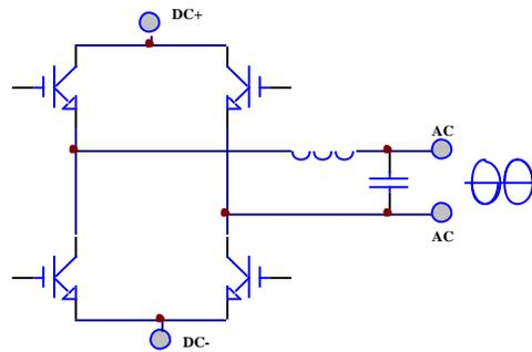
*Figure 1-7 IGBT Inverter*
