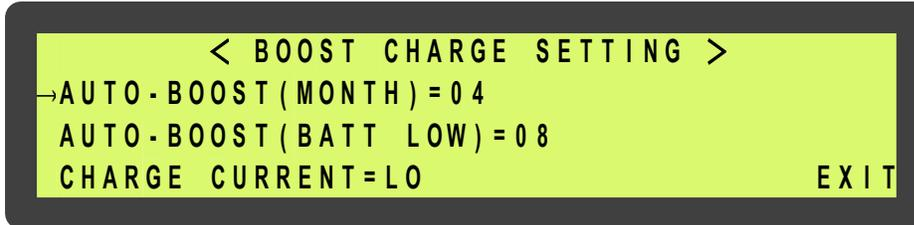
This menu is displayed when the item < BOOST CHARGE > is selected from MENU 5, the PARAMETER SETTING menu. The user can change the charger parameters through this menu. The cursor ( $\rightarrow$ ) can be moved upward by the UP ( $\uparrow$ ) key and can be moved downward by the DOWN ( $\downarrow$ ) key. The selection is confirmed by pressing the ENTER ( $\leftarrow$ ) key. See in the above figure.
