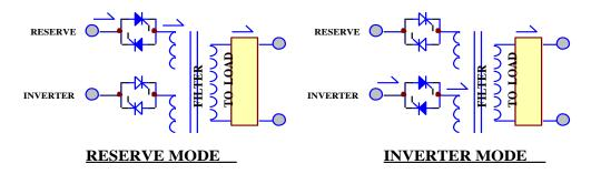
Figure 1-8 Static Switch
