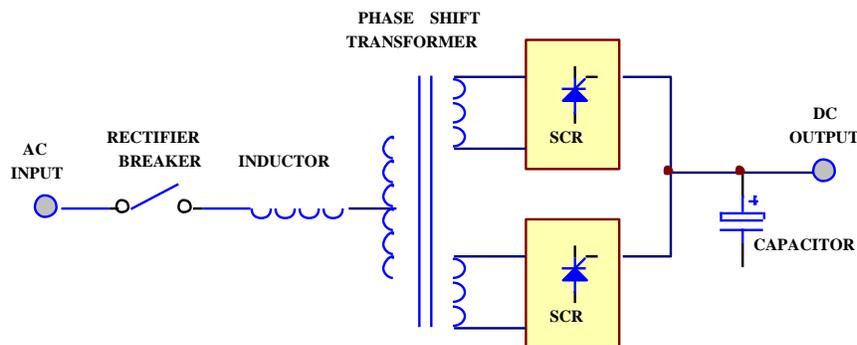
*Figure 1-6 12-Pulse full control rectifier*
