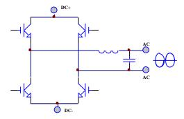
Figure 1-7 IGBT Inverter
