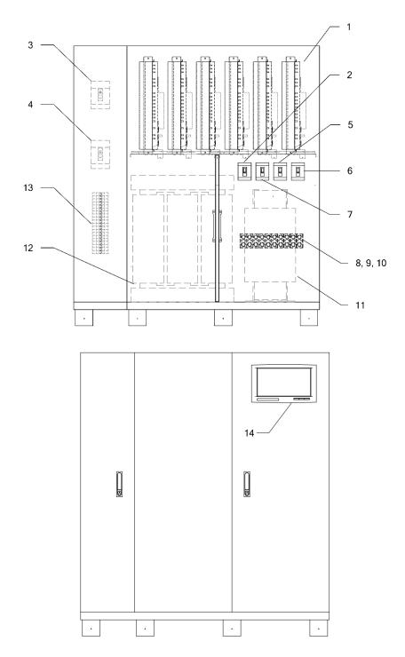
Figure 3-1 Key Components typical location (shown 80-160KVA)
