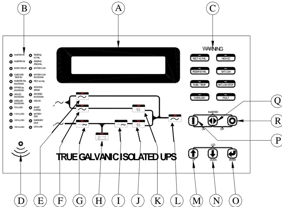
The front panel is located at the front of the PCB holder. It gathers the real time information of the system and shows them clearly to the user. It also provides switches for controlling and setting the unit. Through this panel, the UPS can be not only a stand-alone machine supplying the load, but also closely monitored by the user. Each part of the panel is explained below.
