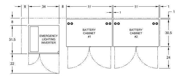
Figure 4-12 Typical system layout (10-60KVA standard battery)
