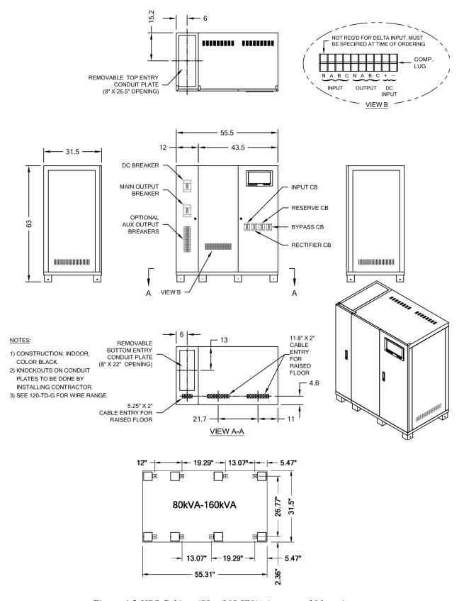
Figure 4-2 UPS Cabinet (80 ~ 160 KVA) Access and Mounting
