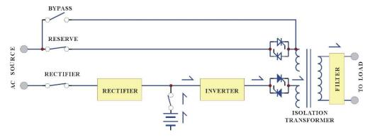
Since the batteries are connected directly to the DC bus, when the AC fails, the batteries change immediately from receiver to donor, supplying energy to the inverter instead of receiving energy from the rectifier. The output AC is not interrupted. Therefore, the load connected to the output is protected.
