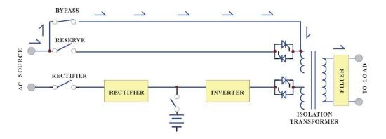
In case of UPS maintenance or battery replacement, and when the load cannot be interrupted, the user can turn off the inverter, close the bypass breaker and then open the rectifier and reserve breakers. The AC output will not be interrupted during manual bypass transfer procedure. Therefore, the maintenance bypass switch keeps continuously supplying power to the load. Electricity will not exist in the UPS except the output transformer, thus ensuring the safety of service personnel.
