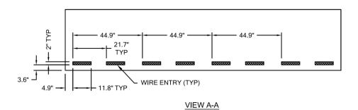
Figure 4-5 UPS Cabinet (500 KVA) Access and Mounting
