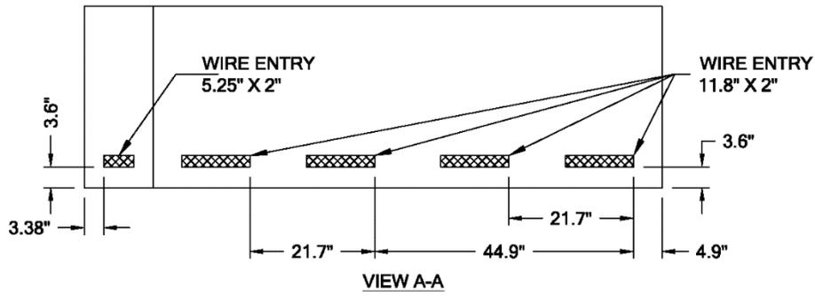
*Figure 4-3 UPS Cabinet (200 ~ 320 KVA) Access and Mounting*
