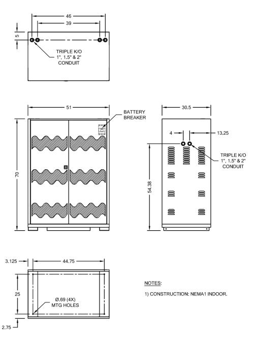
Figure 4-6 Typical Battery Cabinet Access and Mounting
