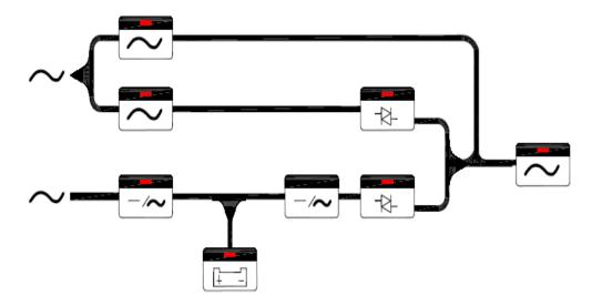
Figure 5-1 Mimic Display under normal operation
