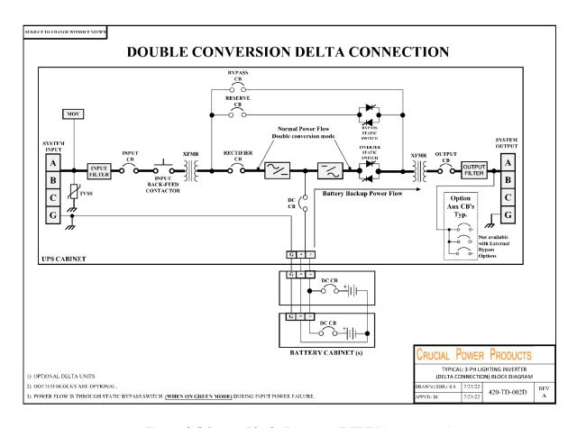
Figure 3-5 System Blocks Diagram (DELTA input power)
