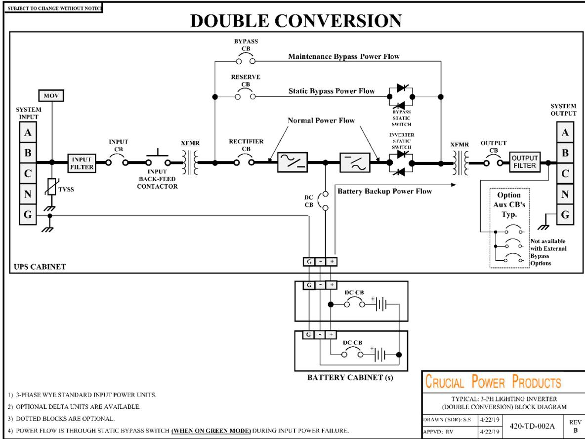
*Figure 3-2 System Blocks Diagram*
