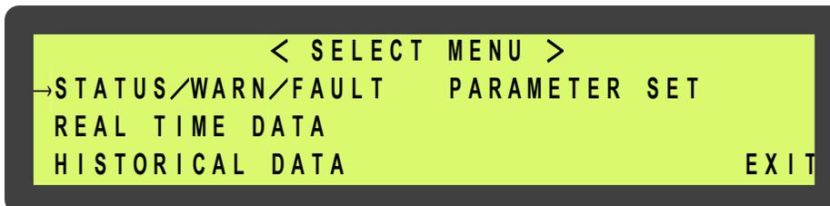
The Select Menu is for the user to select, via the cursor (→), the type of data the user wants to view, such as, inverter on/off, buzzer on/off, charging time and magnitude, date/time etc. The cursor (→)
