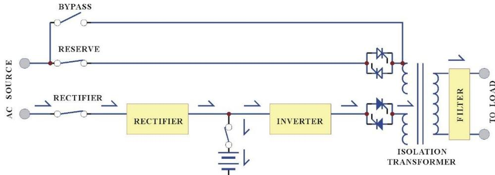
The rectifier converts the AC input to DC power to supply the inverter and charge the batteries simultaneously. All the fluctuations, surges and spikes of the AC input are removed during AC to DC conversion. Therefore, the AC supplied by the inverter is clean and stable.
