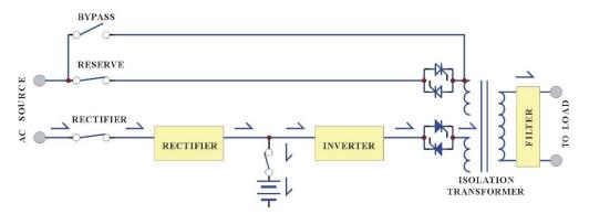
The rectifier converts the AC input to DC power to supply the inverter and charge the batteries simultaneously. All the fluctuations, surges and spikes of the AC input are removed during AC to DC conversion. Therefore, the AC supplied by the inverter is clean and stable.
