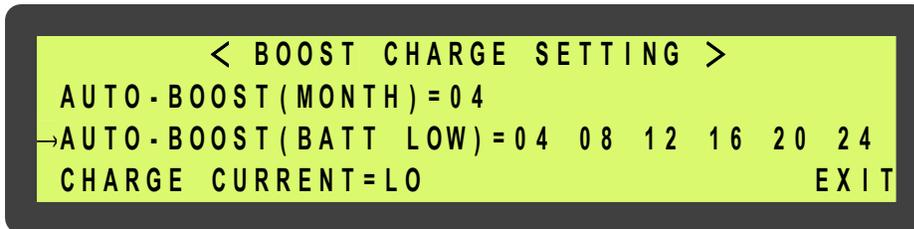
When AUTO-BOOST (BATT LOW) is selected, all the value that can be selected will be shown (04/08/12/16/20/24). The battery will be boost charged every time the battery has been discharged to below 12V/battery or 2V/cell. The boost charge time is set by this row, with the values being “hours”. The current value (or the value being selected) will flash and is confirmed
