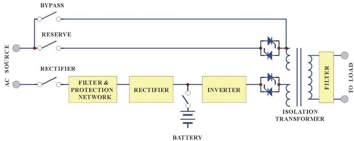
The Unit is composed of input breakers, input filter & protection network, rectifier, battery bank, inverter, static switch, bypass breaker, isolation transformer and output filter. The basic topology is shown in the diagram above. Under normal AC mode, energy from the AC source is converted to DC power and supplied to the inverter to charge the batteries to its full capacity all the time, ready to support the output load in case of AC source failure.
