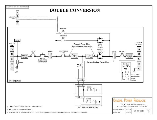
Figure 3-3 System Blocks Diagram (Dual WYE input power)
