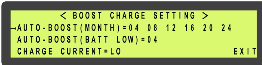
When AUTO-BOOST (MONTH) is selected, all the values that can be selected will be shown (04/08/12/16/20/24). The battery will be boost charged once every month. The boost charge time is set by this row, with the values being “hours”. The current value (or the value being selected) will flash and is confirmed by the ENTER ( $\leftarrow$ ) key. Longer times are selected for bigger batteries according to the needs of the user. Refer to the figure above.
