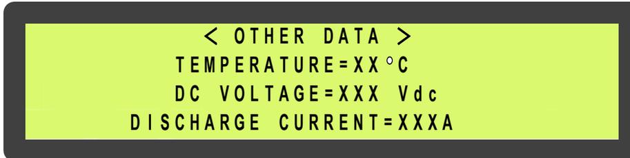
The UP ( $\uparrow$ ) or DOWN ( $\downarrow$ ) keys have no function in this menu. The screen will go back to MENU 3 – the REAL TIME DATA menu, when ENTER ( $\leftarrow$ ) is pressed.
