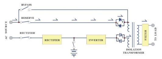
When the inverter is in an abnormal condition, such as over temperature, short circuit, abnormal output voltage or overloaded for a period exceeding the inverter's limit, the inverter will automatically shut down in order to protect itself from damage. If the utility power is normal, the static switch shall transfer the load to the reserve source without interruption of AC output.
