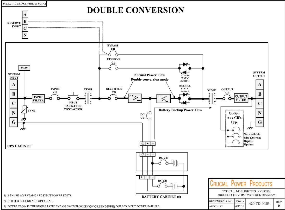
*Figure 3-3 System Blocks Diagram (Dual WYE input power)*
