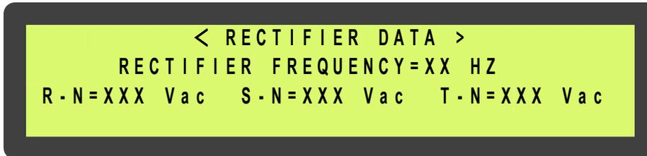
This menu is displayed when <RECTIFIER DATA> is selected from MENU 3 – the REAL TIME DATA MENU. It is a data display menu which shows real time data on the rectifier, such as, RECTIFIER FREQUENCY, R-N/S-N/T-N VOLTAGE, etc. The phase to phase voltage display is also available when input is a delta ( $\Delta$ ) connected source.
