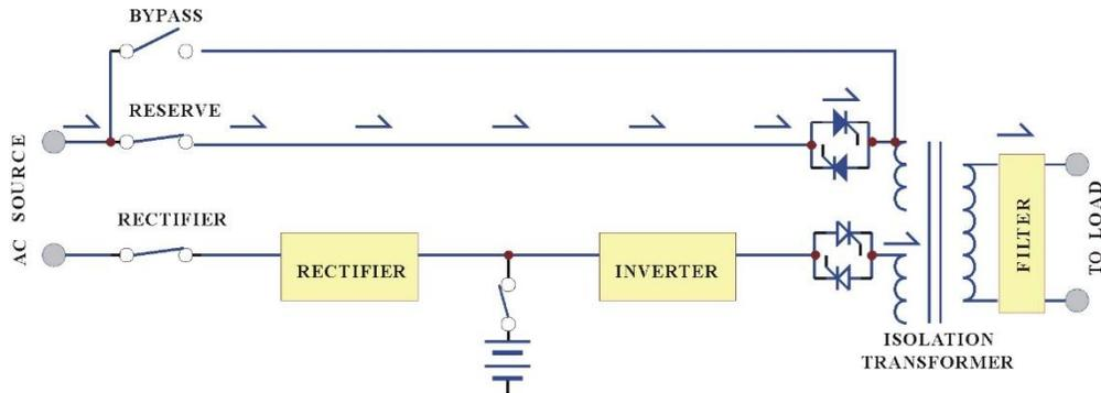
When the inverter is in an abnormal condition, such as over temperature, short circuit, abnormal output voltage or overloaded for a period exceeding the inverter's limit, the inverter will automatically shut down in order to protect itself from damage. If the utility power is normal, the static switch shall transfer the load to the reserve source without interruption of AC output.
