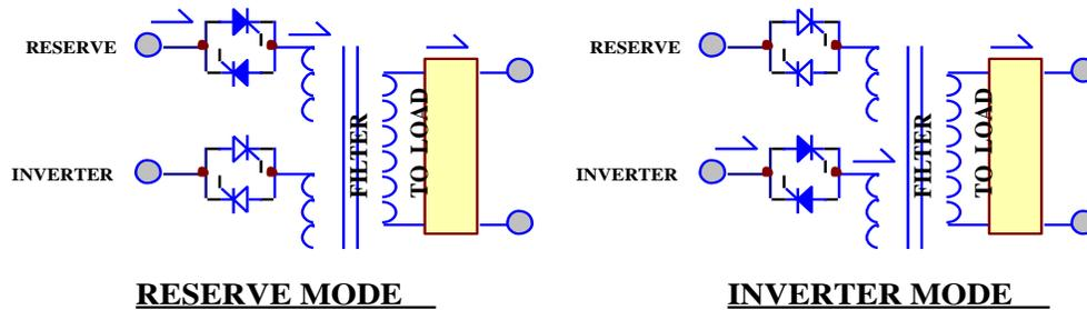
*Figure 1-8 Static Switch*
