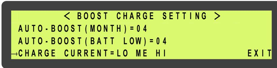
When CHARGE CURRENT is selected, the values that can be selected will be shown (LO/ME/HI). When the batteries are being boost-charged for whatever the reason, the charging current will be limited by a value according the setting in this row. The current value (or the being selected) will flash and is confirmed by the ENTER (←↓) key.
