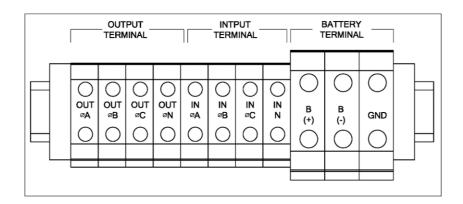
Figure 4-11 Customer Connections to the Input / Output / Battery (DC) Terminal Block (typical)
