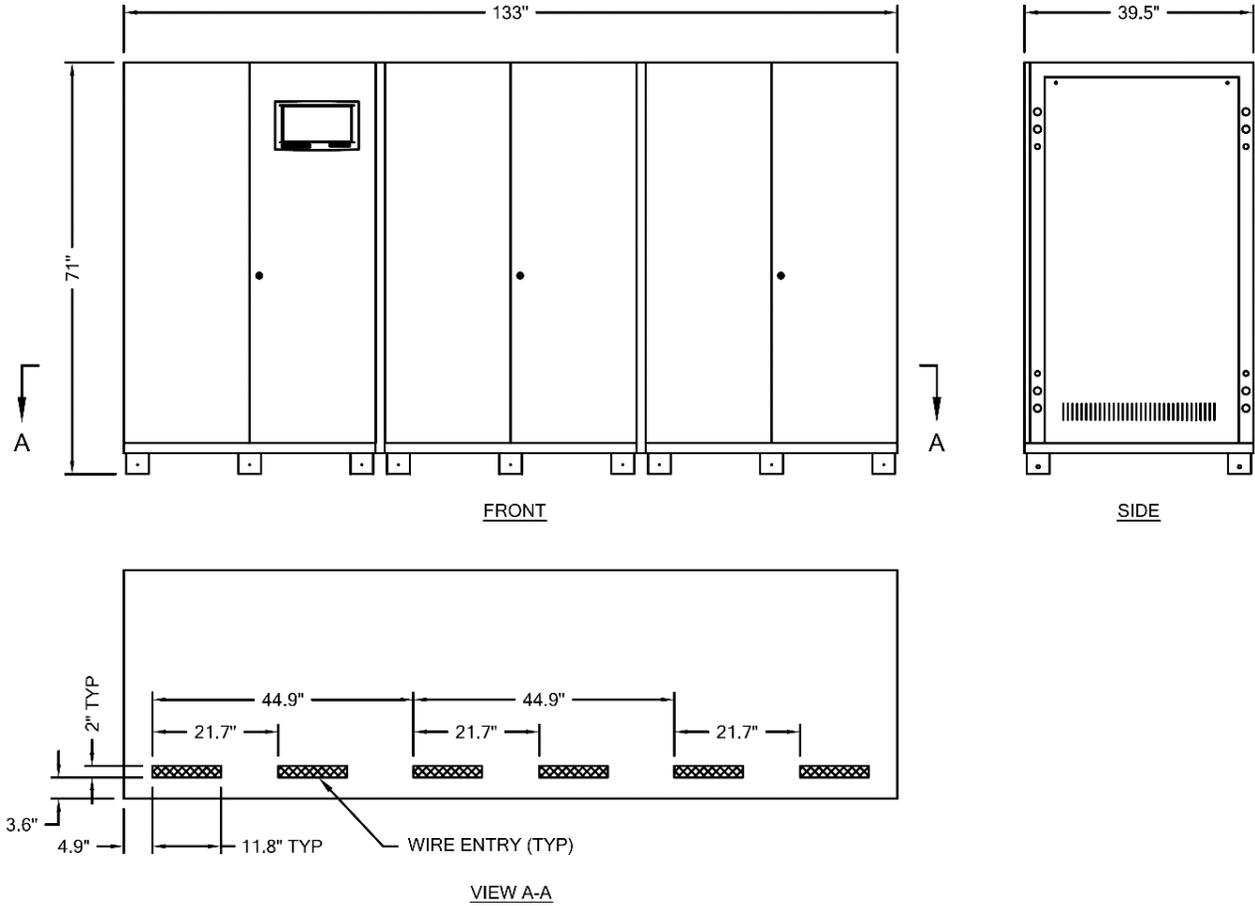
*Figure 4-4 .UPS Cabinet (400 KVA) Access and Mounting*
