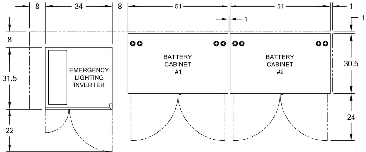
*Figure 4-12 Typical system layout (10-60KVA standard battery)*
