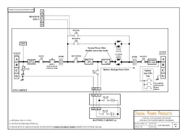
Figure 3-4 System Blocks Diagram (Dual DELTA input power)
