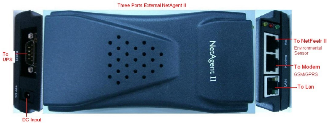
Figure 8-4. Example of Basic NetAgent Mini-external Device
